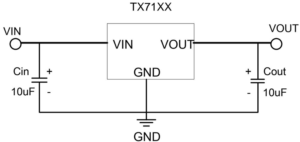
Note1:  $C_{in}=C_{out}=10\mu\text{F}$ . (10uF Electrolytic capacitor is recommended).
